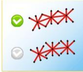
It allows you to fit the programmable stitch on the path, thus presenting a continuity between consecutive programmable stitches, allowing a deformation. If this option is set to No, the figures formed by the programmable stitch are not deformed.
