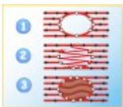
The hole of a complex area section may be: Empty (1) (in which case the rest of the items belonging to the Hole group are disabled), filled with Zig-Zag stitches (2) or with a pattern (3).
