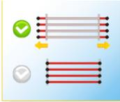
According to several factors, such as the stitch density, the type of fabric, the thread tension, etc., there could be fabric shrinks, causing visible variations in the stitches length.
