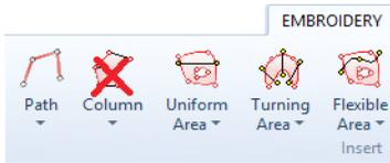
1) Select the Path or Area creation tool and the desired stitch type. Note that with Column section type is not possible apply Auto-complete Mode to geometric figures.
