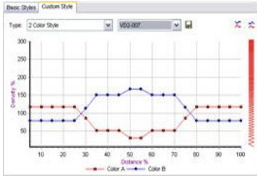
That length is represented by a percentage in the horizontal axis of the density charts, where 0% and 100% are the two ends.
