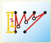
**Level value:** It is the distance of the short stitches, measured in percentage (based on the normal stitches).
