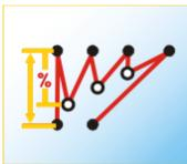
It is the distance of the short stitches, measured in percentage (based on the normal stitches).
