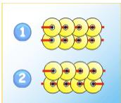
When unchecked, all sequins are placed following the same direction (1). When checked, sequin placement is accomplished following a “go and back” sequence (2)
