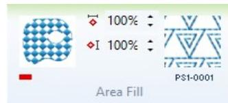
**Description:** The Programmable Stitch may be applied to sections with more complex shapes and holes but will have only one direction and the stitches appearance will not change.
