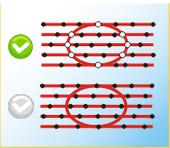
It allows you to specify whether you wish to create stitches on the edges of the holes or not, so as to make them stand out. The options available are Yes or No. You need to add a Border for the main fill to be able to enable this property. It's available on the Borderline tab, inside the Stitch Fill group, on Holes.
