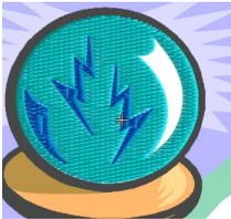
In the left figure you can observe the result, note that the section created contains an empty hole that corresponds to the white area in the ball. The other three have been recognized and filled up with stitches.
