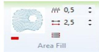
**Description:** This tool fills an area varying the orientation of stitches, adapting them to the direction(s) [either straight or curved] specified for the section.
