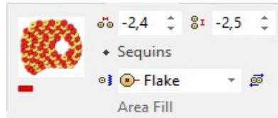
**Description:** This fill type allows you to insert multiple-sequins arranged following a flexible direction (straight or curved). The way the different sequins are placed may be selected using the multi-sequin setup box. See details in Chapter 9, page 18.
