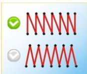
Zig-Zag type fill stitches can be standard (normal) or Z-type, in which stitches are parallel between them and the odd ones produce the forward movement.
