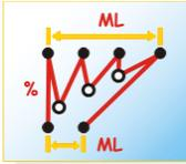
Percentage corresponding to the difference between edges of a section. As from this value intermediate or short stitches will be applied.
