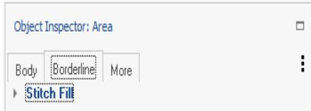
It produces stitches in the border of the section. It is a way of providing the sections with a better finishing, or applying an embossing to the section's outline.
