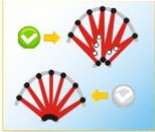
Short or intermediate stitches allow you to compensate the lack and the heaps of stitches. This group of properties is very useful in zones of sharp curves (or differences in lengths) that leave as many spaces without thread as spaces with thread heaps.
