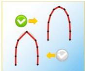
When enabled, Stitch Era adjusts the stitch length in order to minimize the difference between the shape described by the section reference and the shape described by the stitches.
