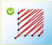
When you activate this control the application will pull the stitches applied to the corners of the section, compensating them automatically. This will allow the optimization of those sections where, due to the geometry of its main reference, the correct finishing of the embroidery is in jeopardy.
