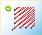
When you activate this control the application will pull the stitches applied to the corners of the section, compensating them automatically. This will allow the optimization of those sections where, due to the geometry of its main reference, the correct finishing of the embroidery is in jeopardy.
